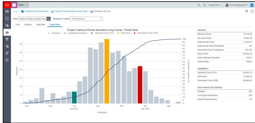
Figure 6B. Monte Carlo-based histograms provide likely project outcomes based on potential risk, not just the planned schedule
